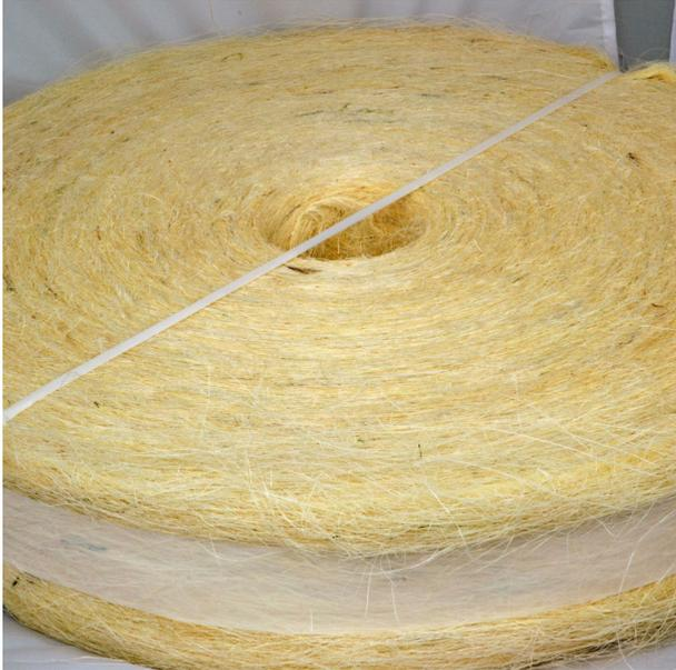
Carded and raw sisal fibre mainly used in gypsum products as a structural element to provide additional reinforcement.
